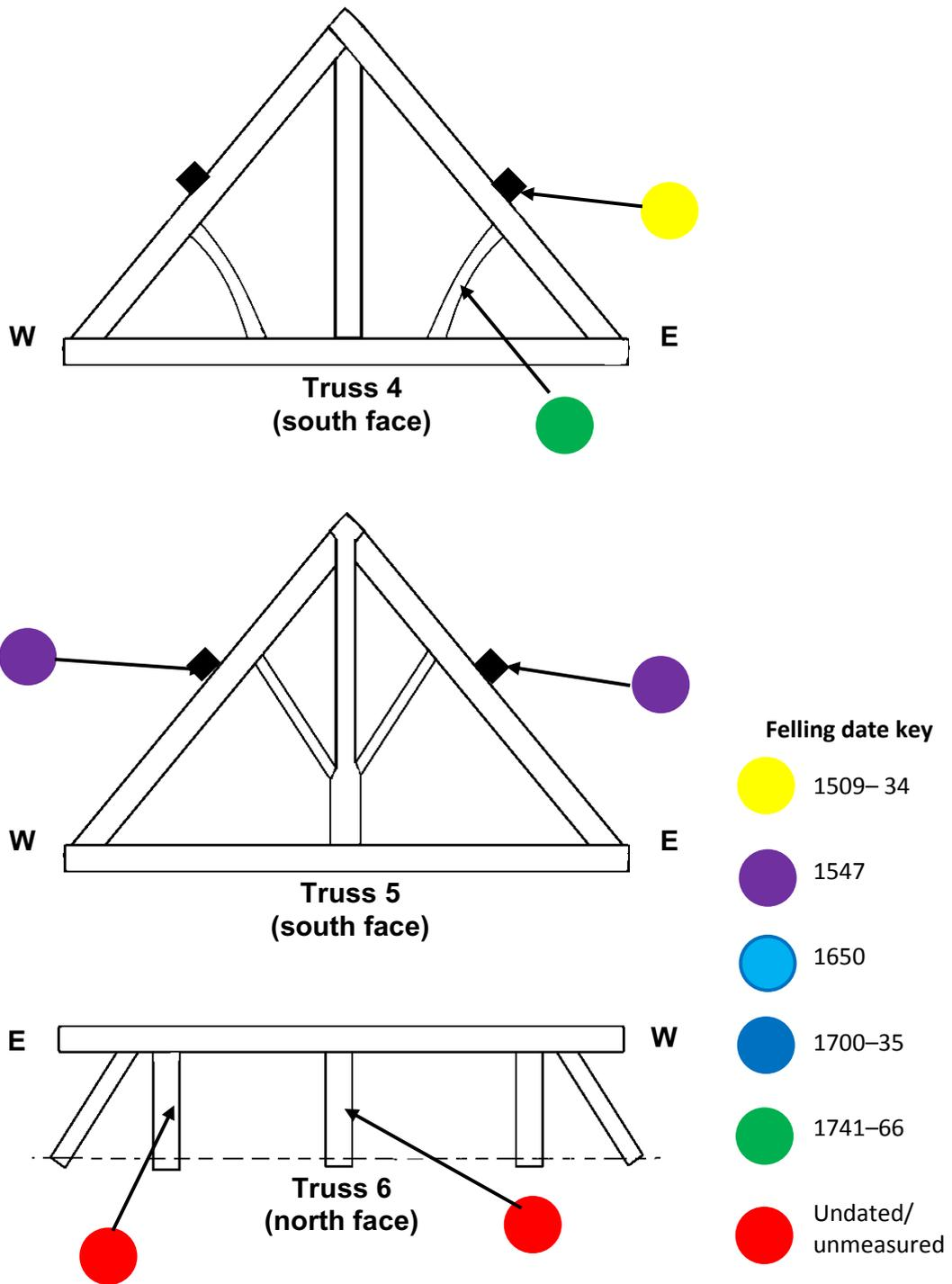
Figures 4a-f. Schematic drawings of the trusses to show, where possible, the sampled timbers, colour coded by felling date/range (where dated) (see also Table 1)
